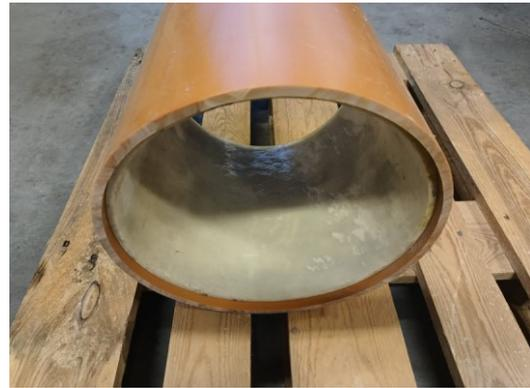
Fig.8. Composite structure –PVC pipe + CIPP liner
