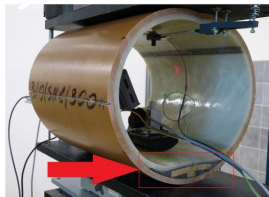
**Fig.9.** Testing of a sample with sediments
