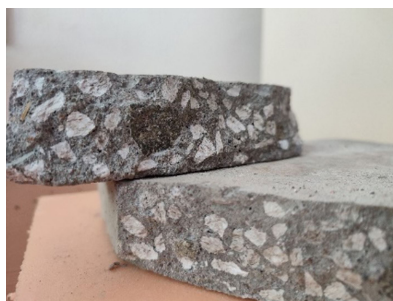
Fig. 1. Cross-section of the exemplary PCM concrete sample
