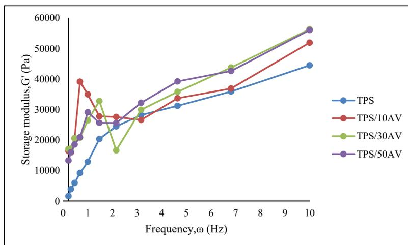
Fig. 3. Storage modulus,  $G'$  of TPS with different concentrations of AV gel
