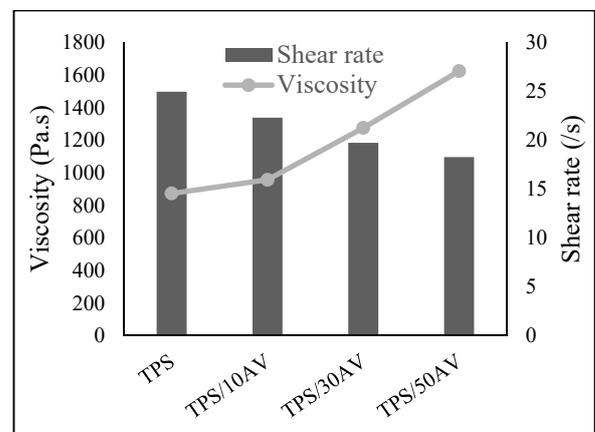
Fig. 2. Viscosity and shear rate of TPS with different concentrations of AV gel
