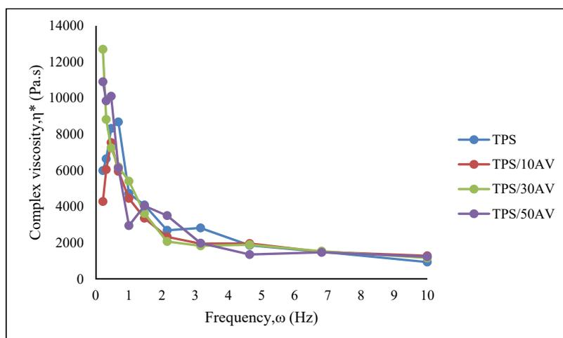
Fig. 5. Complex viscosity,  $\eta^*$  of TPS with different concentrations of AV gel
