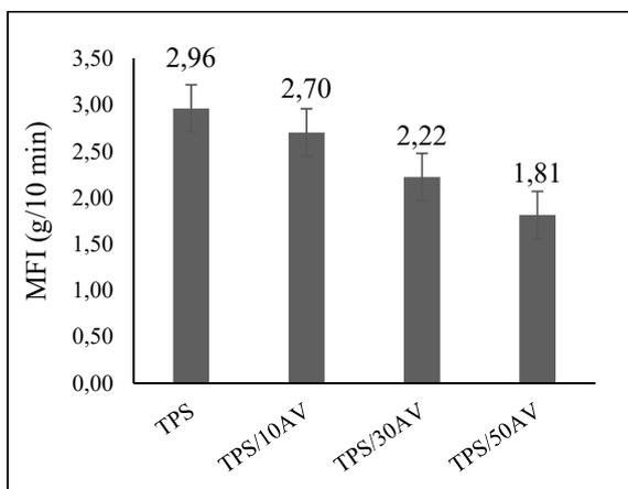
Fig. 1. Melt flow index (MFI) of TPS with different concentrations of AV gel
