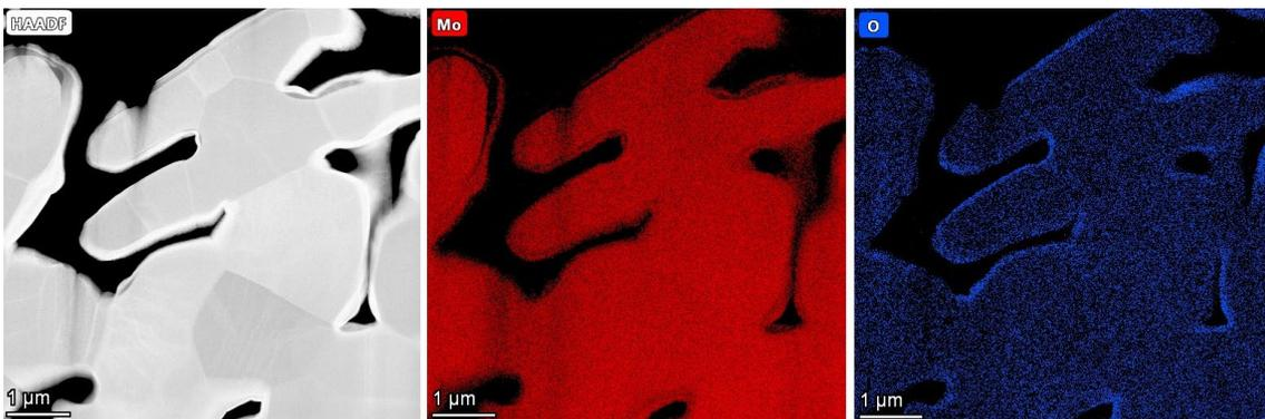
Fig. 3. STEM image & EDS element map distribution of Mo non-spherical powder
