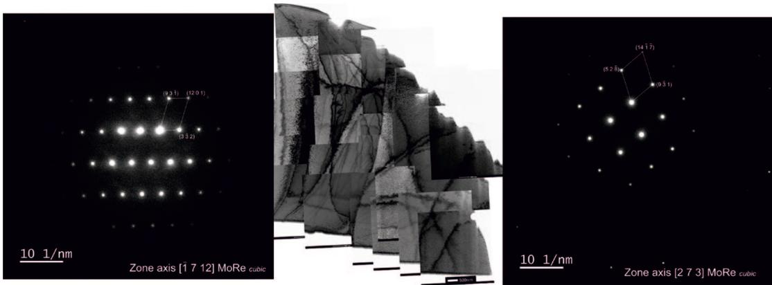
Fig. 12. TEM BF image & SAEDP pattern of Mo-Re spherical powder
