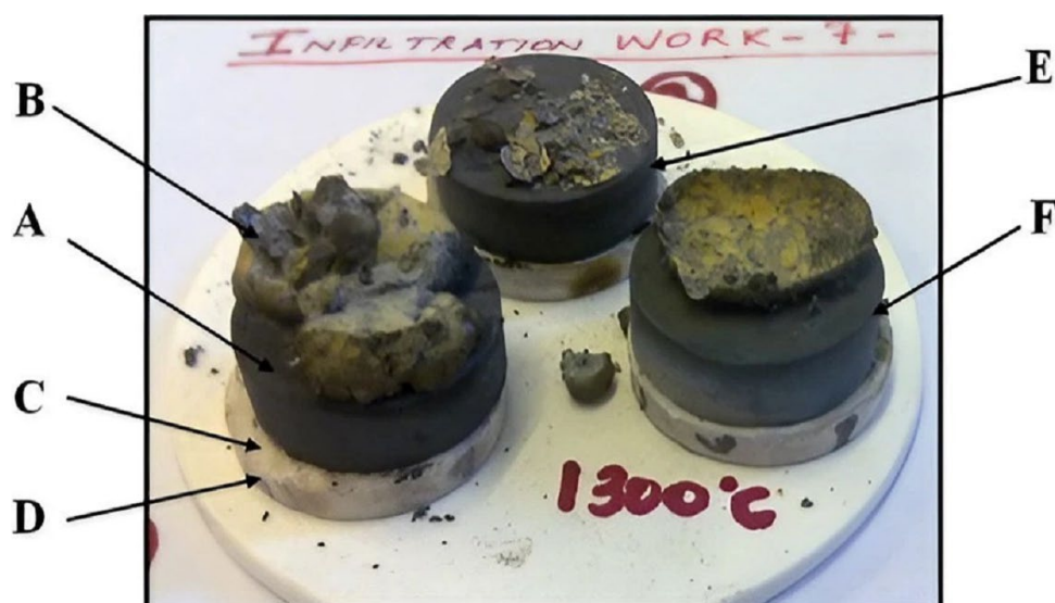
Fig. 8. Results of RMI process accomplished under 1300°C (A) non-infiltrated preform of B_4C ; (B) on top of preform remnants of the Si-Al alloy; (C) thin layer of aluminium oxide (D) aluminium oxide plate; (E) and (F) completely infiltrated composites
