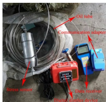
Fig. 14. Kse-1 mining intrinsic safety digital display borehole stress meter
