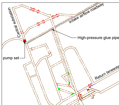
Fig. 8. Location diagram of underground pump set
