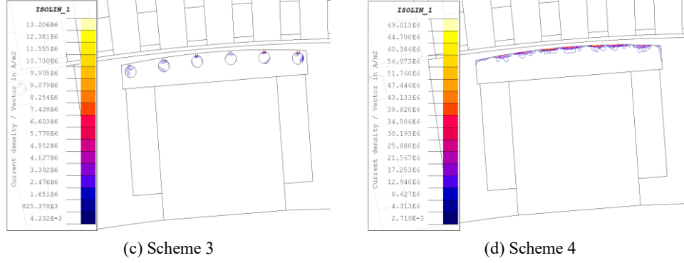
Fig. 11. Rotor pole face eddy-current density for four damping winding configurations
