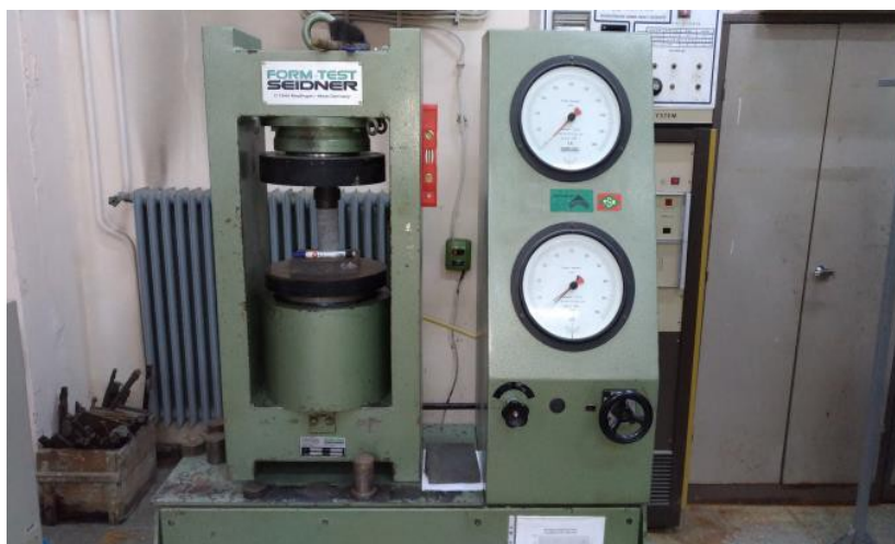
Fig. 2. Hydraulic press used for the uniaxial compressive strength test
