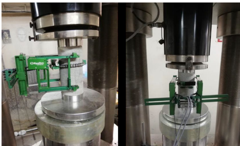
Fig. 3. Setup for the deformability tests used in determining static elastic constants
