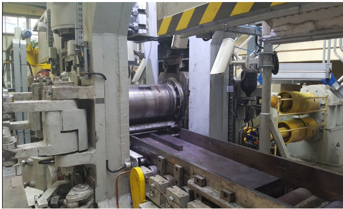
Fig. 1. Single-pass hot rolling of small-sized samples in the LPS/B line
