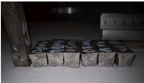
Fig. 8. Results of the Althoff-Radtke test: From left, reference sample; 0.15 % Fe-Nb; 0.31 % Fe-Nb; 0.77 % Fe-Nb; 1.08 % Fe-Nb; 1.54 % Fe-Nb; 2.31 % Fe-Nb.
