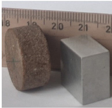
Fig. 5. Samples for density measurements using the spring balance: sandstone cylinder on the left and aluminium cuboid on the right.
