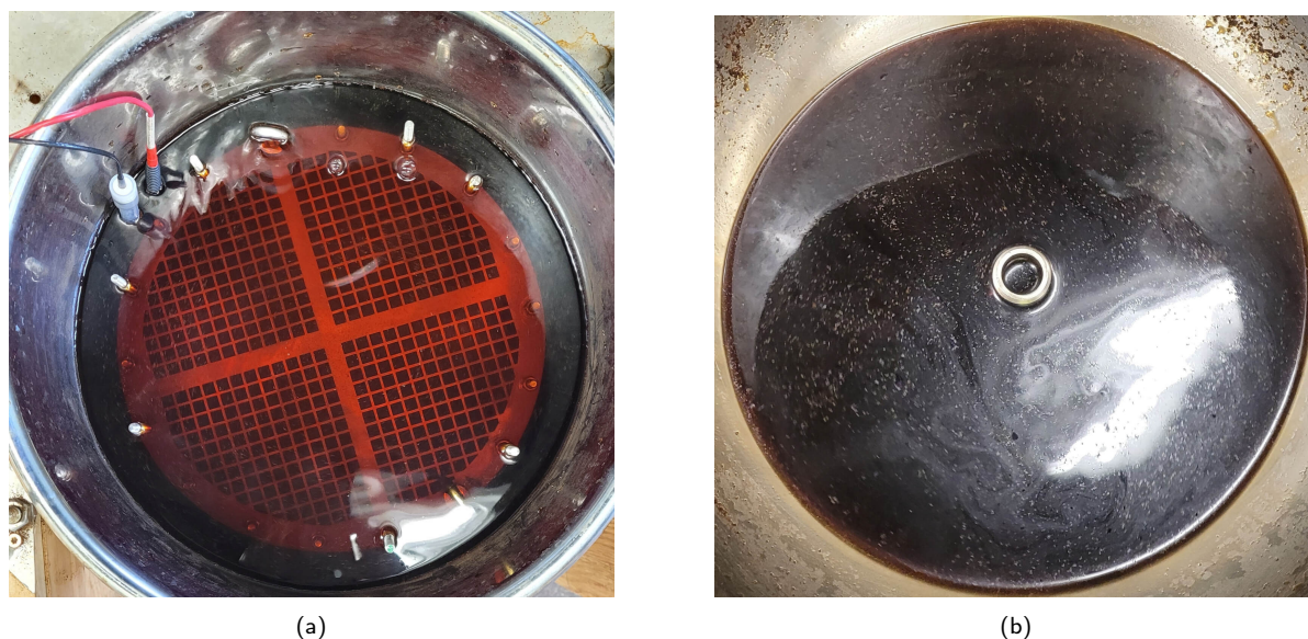
Figure 7. Interior view of the tank with type II basket (Test C): a) soaking of the basket in the extract from Test B ( t_0 = 5 min), b) extract after completion of the experiment ( t = 45 min).
