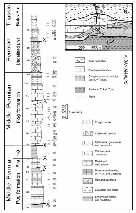
Text-fig. 4. Stratigraphic log of the Permian of Pog, measured along the road. To save space on the drawings the label AA (Albanian Alps) is omitted. Geological map of the area north of the village of Pog is inserted in upper-right corner. The road curves mentioned in the text where the first *Meandrospira pusilla* (Ho, 1959) have been obtained from the Boks Formation, are shown on the map
