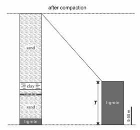
Text-fig. 7. Conceptual model of Hager et al. \$\( (1981) \) method applied to estimate the compaction ratio for lignites from Lower Rhine Basin in northwest Germany.
