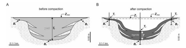
Text-fig. 8. Conceptual model of Widera's (2002) and Widera et al. s (2007) method applied to estimate the compaction ratio for lignites from sedimentary basins in central Poland. Redrawn with modification from Widera (2002) and Widera et al. (2007)
