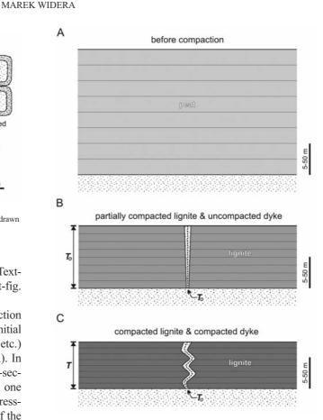
Text-fig. 5. The use of clastic dykes to calculate the compaction ratio. Visualization based on the concepts of various authors
