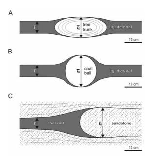
Text-fig. 2. The use of 'fish-tail' forms to calculate the compaction ratio.
