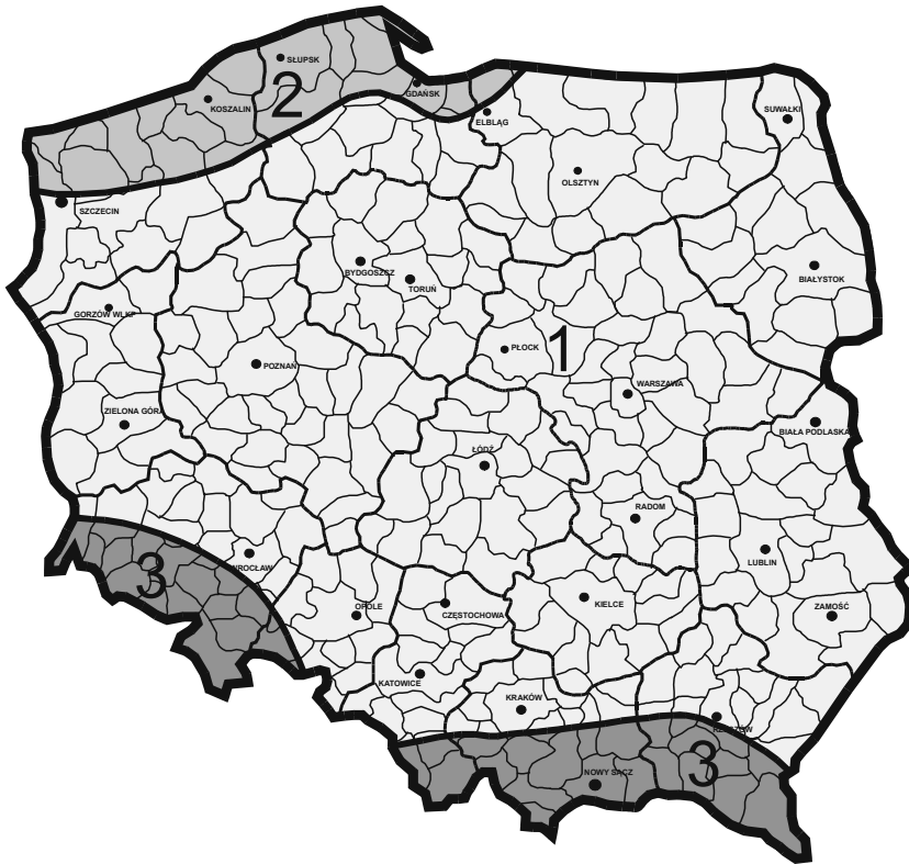
Fig. 28. Wind loading zones in Poland (in conjunction with Table 3 and 4) according to PN-EN 1991-1-4:2008
