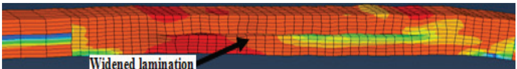
(g) Wire specimen with 30mm lamination located 2.5mm below wire's top surface
