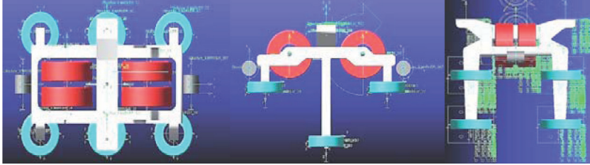
Fig. 2. The bogie subsystem modeled in the MBD tool, different 2D views of the 3D model
