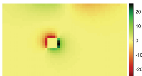
Fig. 3. J_x component of eddy currents density ( \text{mA}/\text{m}^2 ) in the object with non-conductive inclusion
