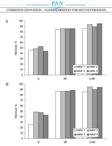
Fig. 3. Comparison of zearalenone (A) and α-zearalenol (B) removal during ozonation (O), nanofiltration (NF) and integrated system (O-NF)
