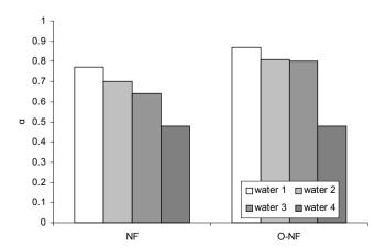
Fig. 4. Relative volume permeate flux α determined during nanofiltration carried out as a single process and in the system integrated with ozonation
