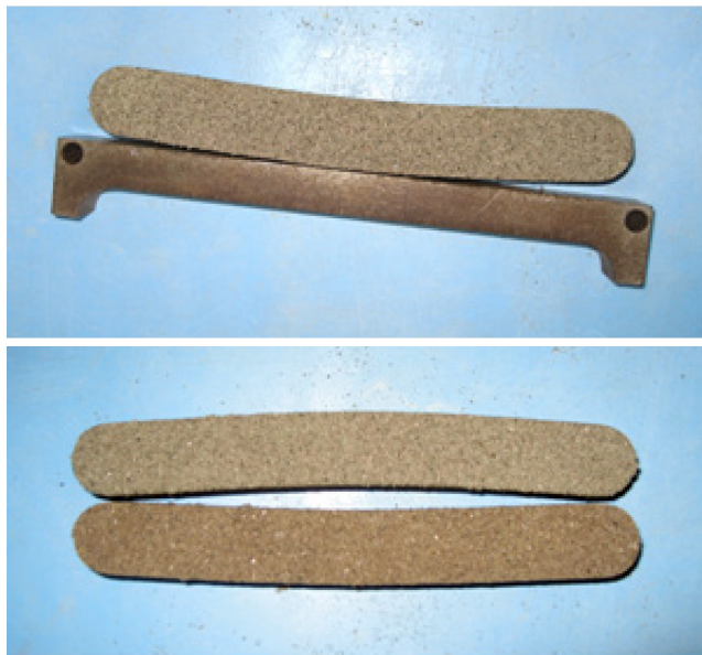
Fig. 4. Plastic state of self-setting mixtures in water presence (1 %) after 1 h hardening (ester HX60)
