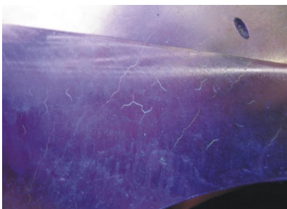
Fig. 1. Net of cracks on test casting surface
