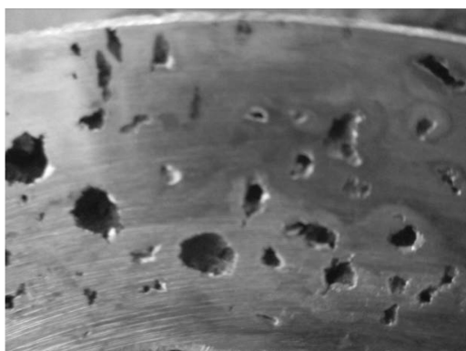
Fig. 1. Gaseous porosity in the copper cast section
