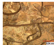
Fig. 29. Sample 5 Metal matrix in EN-GJL-250 cast iron, 500x, ordinary light
