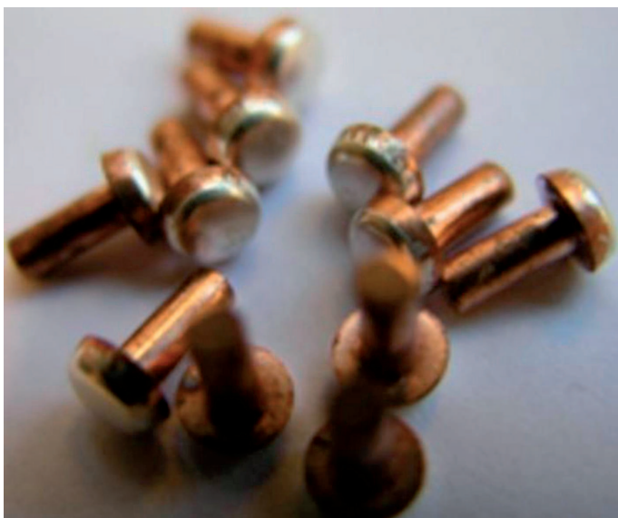
Fig. 5. Bimetallic contact rivets made from the Ag-Re10 contact material
