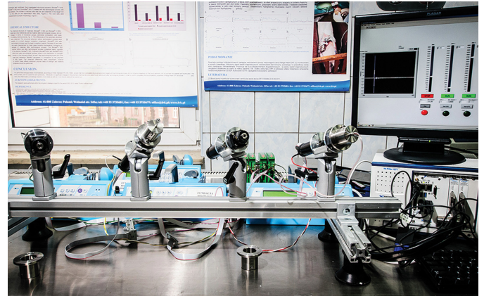
Fig. 3. The physical model for blood rotating with different rotational velocity over a biomaterial surface
