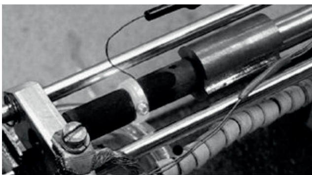
Fig. 2. Actual view of device used for resistance welding without a glass tube used for introduction of argon.
