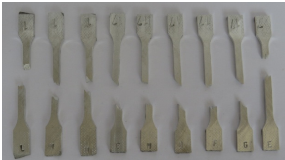
Fig. 14. Test specimens after fracture
