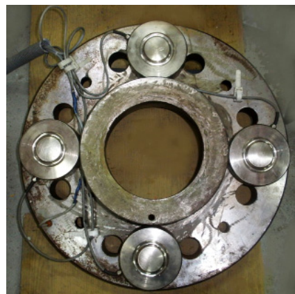
Fig. 4. Measuring disk with distributed force sensors (photo: K. Skrzypkowski)
