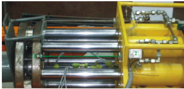
Fig. 6. Cable encoder installed on the HUK machine (photo: K. Skrzypkowski)
