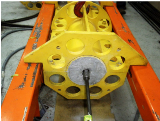
Fig. 3. Dual bushings – rock bolt mounted in a concrete block (photo: K. Skrzypkowski)
