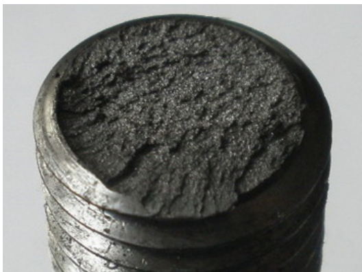
Fig. 11. View of rod surface after rupture (photo: K. Skrzypkowski)
