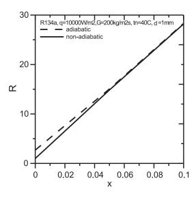
Figure 1. Sample prediction of non-adiabatic effect in bubbly flow, tn – inlet saturation temperature, d – diameter.
