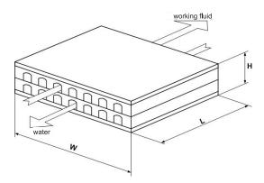
Figure 3. Two layers of the microchannel heat exchanger.
