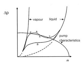
Figure 2. Characteristics of the pump and channel featuring the boiling fluid — Ledinegg instability [6].
