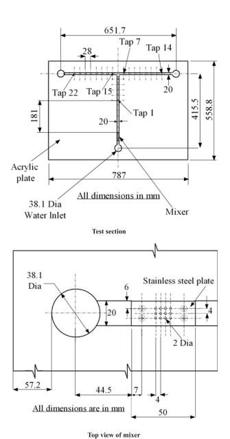
Figure 2. Details of the test section and the mixer.
