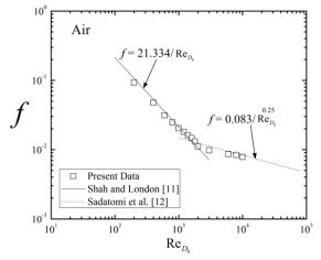
Figure 3. Single-phase air friction factor.
