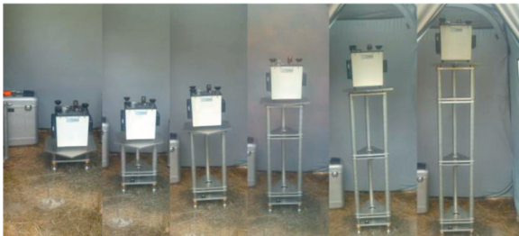
Fig. 20. The stand constructed by WUT (left) and IGK (right) for vertical gravity gradient determination at field station and laboratory station, respectively
