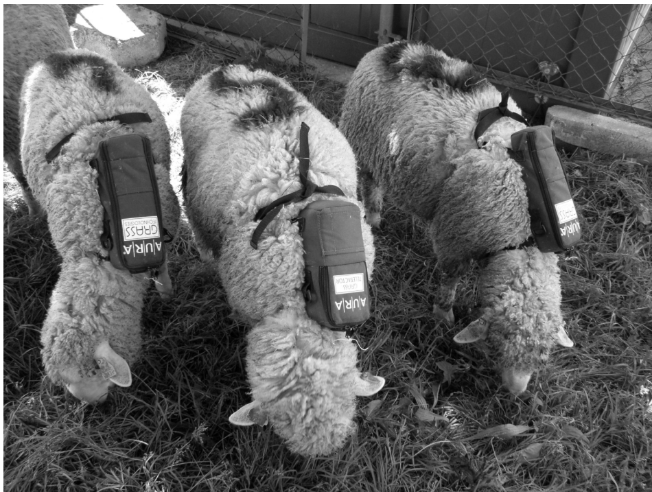
Fig. 4. The ambulatory system (Holter EEG) and its installation possibility on the back of the experimental animals.
