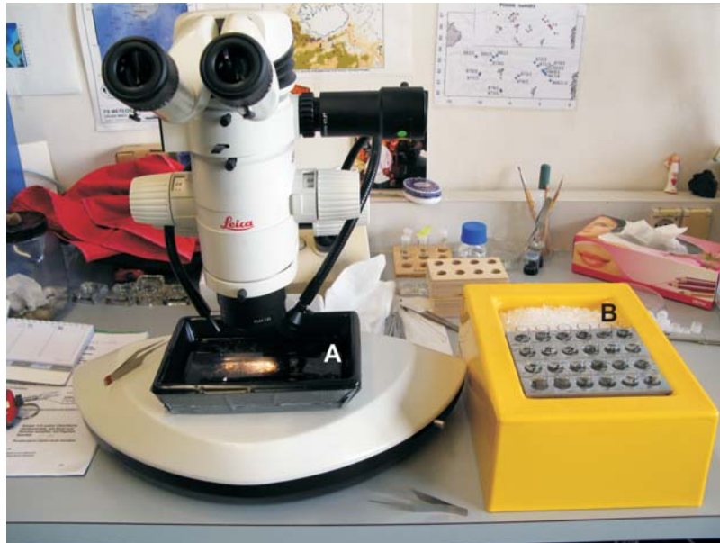
Fig. 2. “Sorting on ice” set-up. Keeping the samples cool throughout the whole range of processes, from sampling until the extraction, seems to be beneficial for generating high-quality DNA sequences. A. Ice dish used to cool the samples during the sorting process. B. Ice bath with metal racks holding taxon vials.
