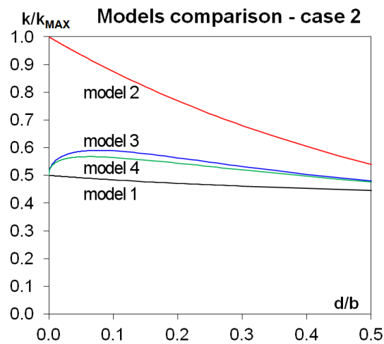
Figure 12: Models comparison for high density PE (polyethylene) and ethanol, B = 0.682 .
