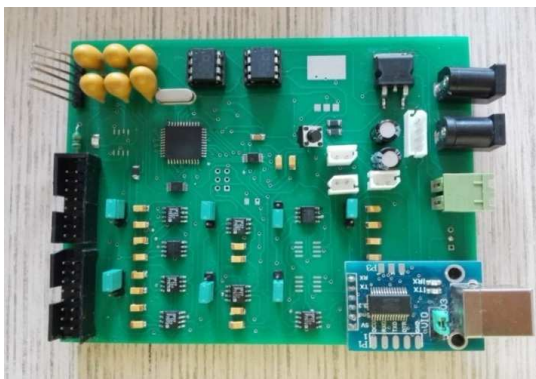
Fig. 8. The circuit board of the electrical impedance spectroscopy system.
