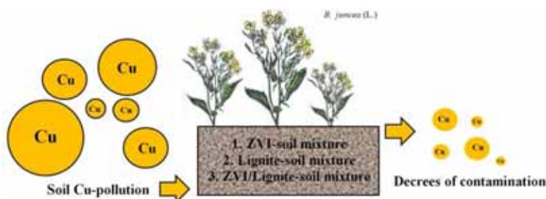
Fig. 1. Concept of co-remediation of Cu-polluted soils with ZVI and lignite; source: own elaboration
