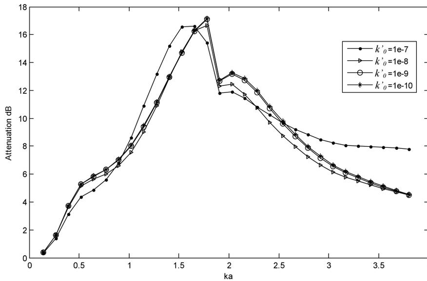
Fig. 11. Effect of the thermal permeability  $k'_0$  [ $m^2$ ] of the porous material on the acoustic power attenuation of the lined duct element.
