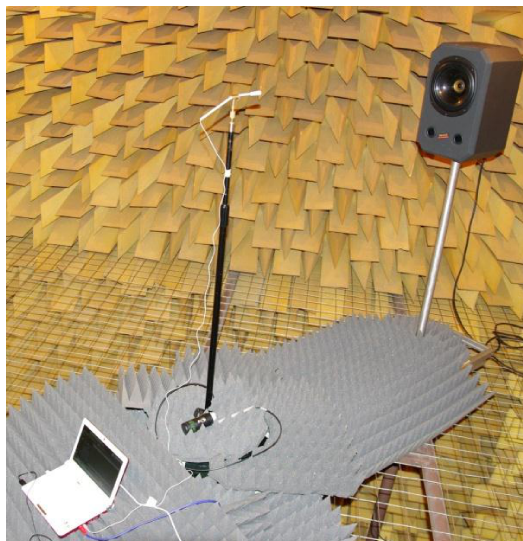
Fig. 6. Overall view of the measurement setup in the anechoic chamber.
