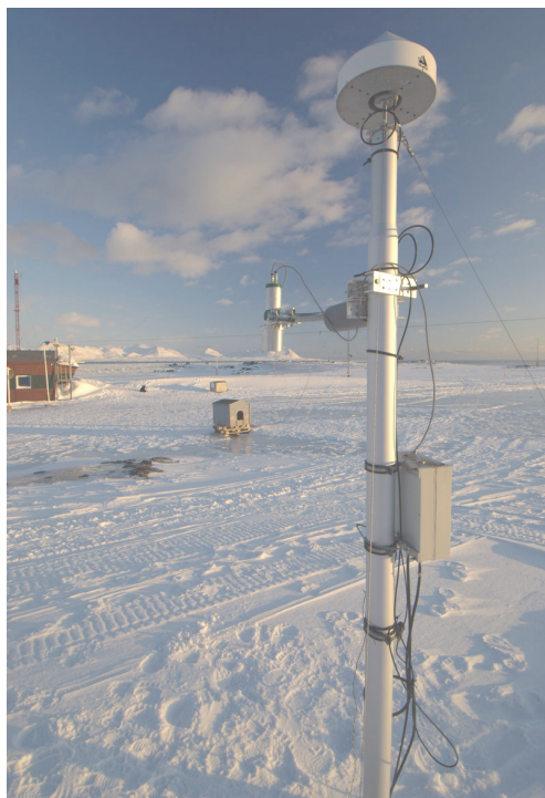
Fig. 11. Ultrasonic instrument measuring snow layer thickness mounted on a meteo mast during research on Spitsbergen.
