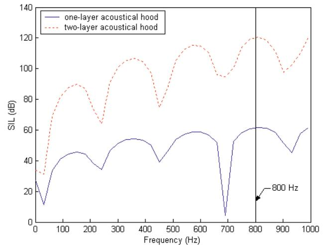
Fig. 9. The optimal  $SIL$  curves with respect to one-layer and two-layer acoustical hood [optimal design set of a one-layer acoustical hood is ( $d_1 = 0.019781$ ;  $h_1 = 0.73809$ ;  $\eta_1$ )] (targeted tone: 800 Hz).
