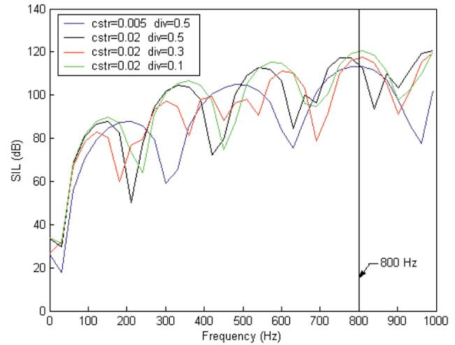
Fig. 8. The  $SIL$  with respect to frequencies at various AIM parameters ( $cstr$ ,  $iter$ ) (targeted tone: 800 Hz).
