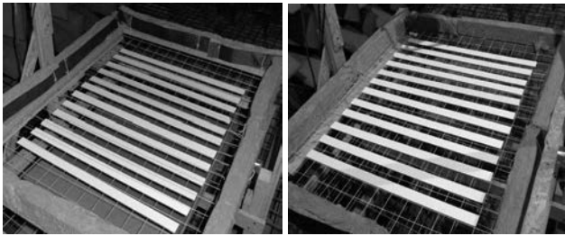
Fig. 4. Studied reflecting structure ( \mu = 0.6 , \varepsilon = 70 ) positioned over the reflecting plate simulating the ceiling and without this plate.
