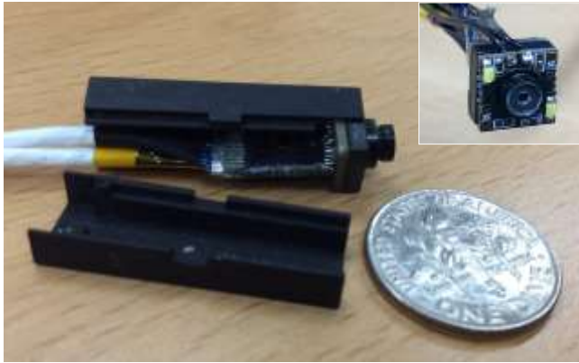
Fig. 4. Photo of the manufactured camera head. The inset show the illumination unit mounted on the holder.
