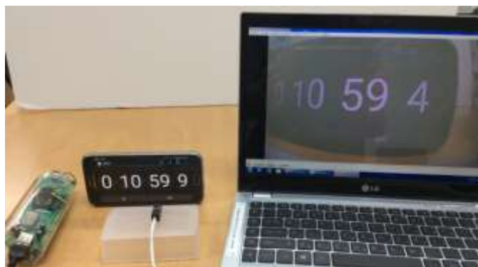
Fig. 12. Latency measurement in Wi-Fi communication mode
