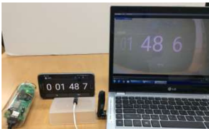
Fig. 11. Latency measurement in UWB communication mode.
