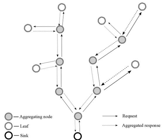
Fig. 1. The tree structure of the aggregation network
