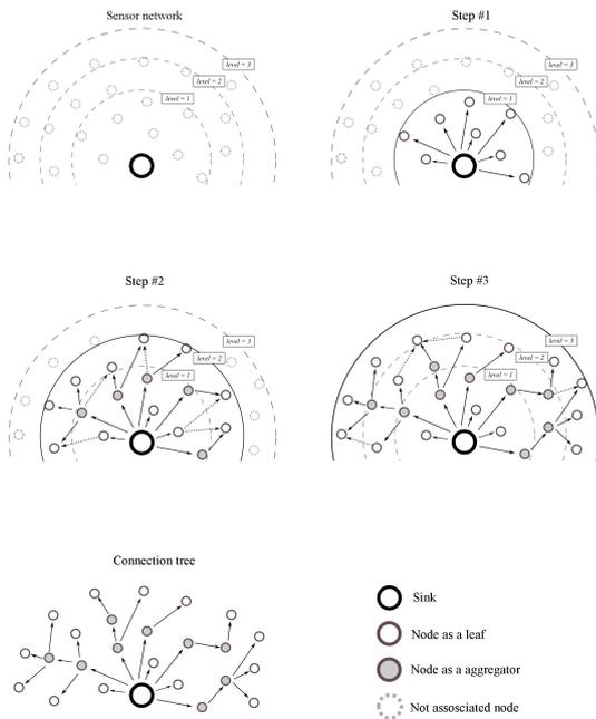
Fig. 2. The tree structure creation process
