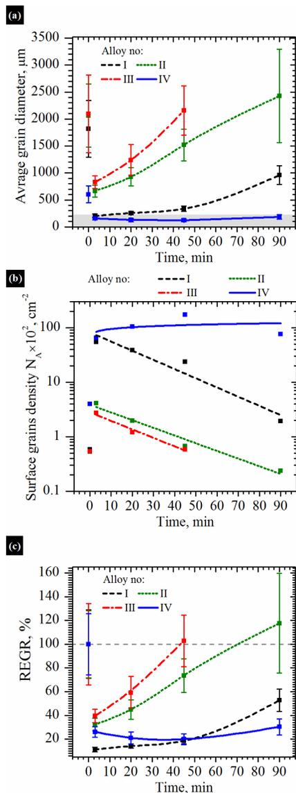
Fig. 3. Variation in the average grain diameter (a), the surface density of  $\alpha(\text{Al})$  grains (b) and the relative effectiveness of grain refinement (c) as a function of time, from the addition of the master alloy
