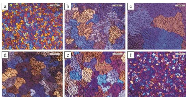
Fig. 2. Macrostructures: (a) alloy I after 3 minutes of grain refinement (b) alloy III after 3 minutes of grain refinement, (c) alloy II in its initial state, (d) melt II 3 minutes after grain refinement (e) alloy IV in its initial state, and (f) alloy IV after 3 minutes of grain refinement
