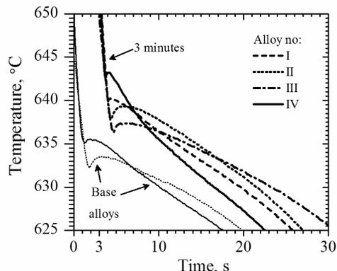
Fig. 1. Cooling curves recorded for base alloys (no. I and IV) and after 3 minutes from the introduction of master alloys (I to IV)
