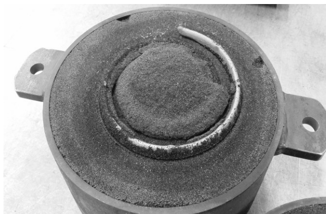
Fig. 1. Discolouration of chromite sand base (bonded with sodium silicate) in the layers adjacent to iron casting
