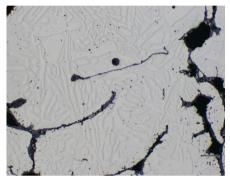
Fig. 3. The film an inclusions from the sample 1.4517 (magnification 100x)
