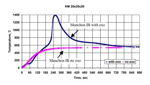
Fig. 9. Comparison of temperature curves recorded for the KM sleeves material with the exo effect and without this effect
