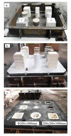
Fig. 1. Selected stages of producing a mould containing tested materials: iso-exo sleeves and insulating bricks.
