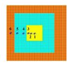
Fig. 11. 3D discretization of specimen (yellow, 1,2,3) – furnace (blue, 3,4) – ambient (orange, 6) layout and posi- tions of virtual thermocouple sensors (1 to 5), NF&S CV 6.0
