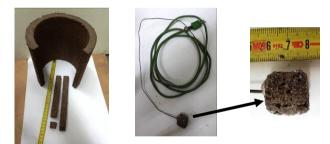
Fig. 7. Method of cutting a 20x20x20 mm specimen out of a sleeve and installation of a sheathed K thermocouple in its geometrical center
