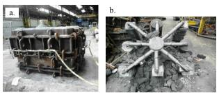
Fig. 2. View of a mould ready for pouring, with visible group of compensating cables (a) and castings after knocking out (gating system side). Total mass of castings with the gating system – approx. 2700 kg
