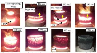
Fig. 4. Sequence of selected steps of exo reaction progress for isoexo sleeve diam.120mm placed on a liquid cast iron plate specimen (PS). The arrows show the direction of the exo reaction
