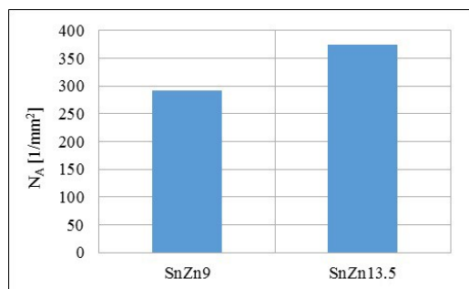
Fig. 4. Comparing the average number ( N_A ) of Zn-rich precipitates observed in eutectic SnZn9 alloy and in hypereutectic SnZn13.5 alloy
