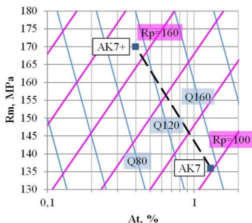
Fig. 7. Nomogram of Drouzy et al. [14] for the quality evaluation of the AlSi7Mg0.3 -type alloys with the use of the quality index Q, on the background of the plasticity isolines Rp
