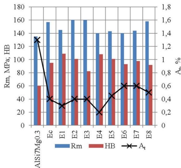
Fig. 3. Mechanical properties of the AlSi7Mg0.3 alloy without the additions and with the alloy additions AlSi7Mg0.3+(CuNiCrVMoW)
