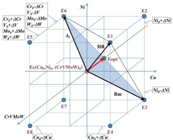
Fig. 4. Directions of the vectors of the Rm, A<sub>t</sub>, HB change gradient – selection of the optimal composition of the Eopt silumin (AK7+) AlSi7Mg0.3+4% Cu+2% Ni+0,1% (CrVMoW) each
