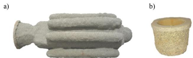
Fig. 1. Ceramic mould for strength sample casting (a) and ATD10C-PL sampler (b)
