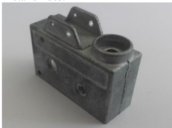
Fig. 1. View of surface faults on the tap casting used on the housing of micro switch
