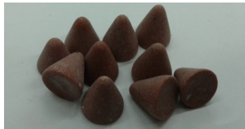
Fig. 2. Polyester abrasive fittings PB 14 KT
